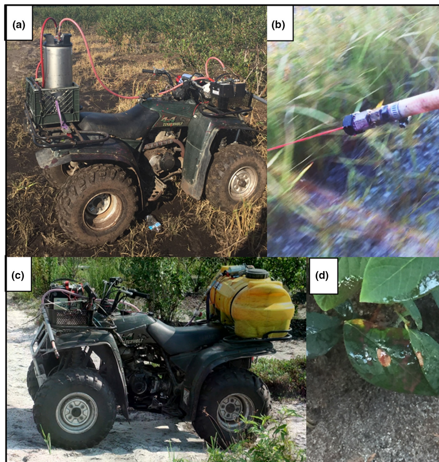
FIGURE 1 Field applications of HOOK SWD in commercial blueberry farms were made using a customized 4-wheel-drive ATV (a, c), with type D2 or D3 orifice nozzles (b) to achieve a consistent spray flow. The sprayer was calibrated to deliver 3.75 L/ha at 35 psi (2018) or 6.25 L/ha at 40 psi (2019) of HOOK SWD. HOOK SWD applications were aimed at the lower third of blueberry bushes to avoid contamination of harvestable fruit (d). [Colour figure can be viewed at wileyonlinelibrary.com ]
