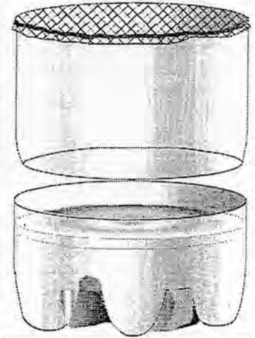
Figure 10. A mosquito emergence cage made from a 2-liter soft-drink bottle. Cut around the circumference to detach the "larval bath" and cut off the top, a little above the turning point. Invert the top and fit it into the bottom. Glue a disk of screening to the "top" (bottom of the top)!
