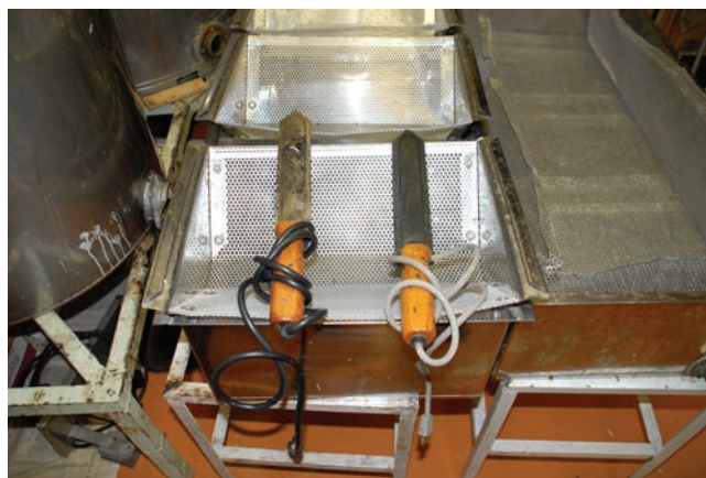
Figure 3 – Hot electric knives. These have a built-in thermostat that helps keep the knives from overheating and burning the honey and wax. Photograph, University of Florida.
