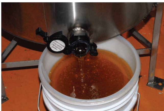
(l) Figure 11 – Honey passing through a filter, into a bucket. This particular filter has two mesh sizes. The upper mesh filters out the large debris while the lower mesh filters out the smaller debris. (r) Figure 12 – Stainless steel settling tanks. Photographs, University of Florida.
