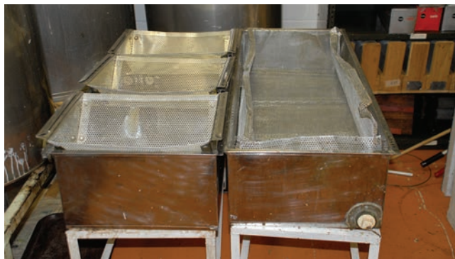
(l) Figure 6 – Uncapping bucket. This bucket would be better if there were a screen on the bottom to allow the honey to drain away from the cappings. (r) Figure 7 – Stainless steel uncapping tanks. The screen mesh allows the honey to drain from the cappings. Photographs, University of Florida.
