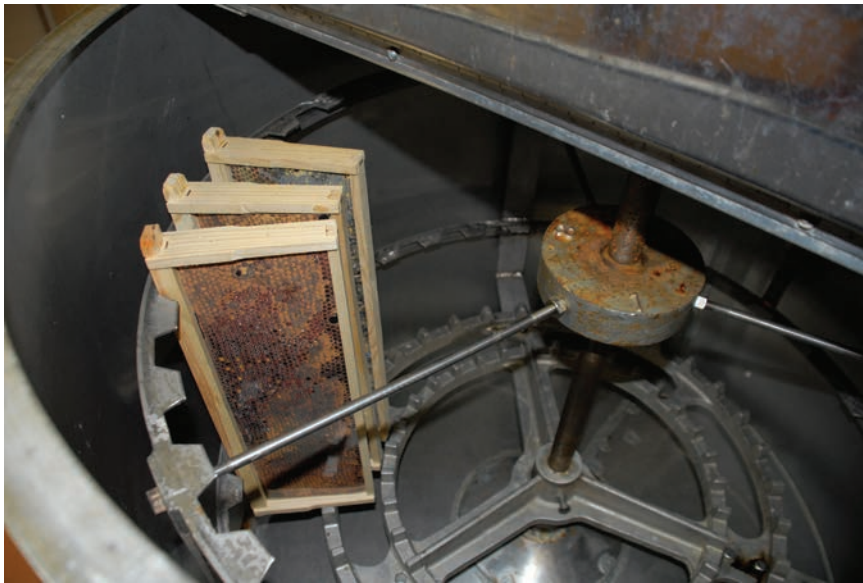
Figure 10 – Frames placed into an extractor. This extractor is able to extract both sides of the frames at once. You can know this by seeing the frames' arrangement in the extractor. When frames lie perpendicular to the center of the extractor, the extractor can extract honey on both sides of the combs at once. When the face of the comb lies parallel to the center and walls of the extractor, the extractor can only extract one side of the frame at a time. Photograph, University of Florida.
