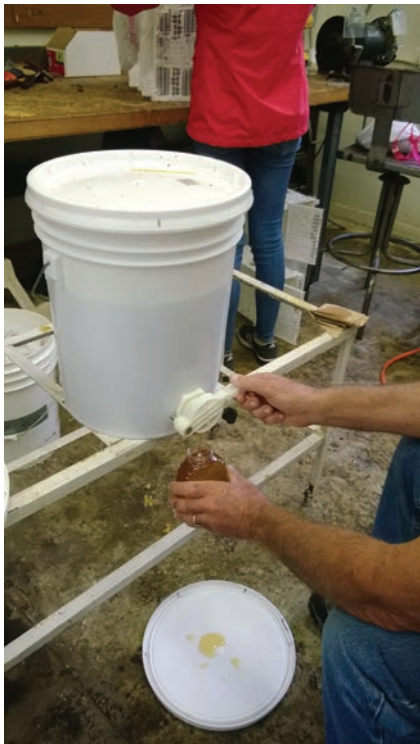
Figure 13 – A 5 gallon (~20 l) bucket used as a settling tank. Just about any container can be made into a settling tank. The honey gate at the bottom of the bucket can be purchased separately from beekeeping supply companies. They can be attached to many types of containers. Photograph, University of Florida.
